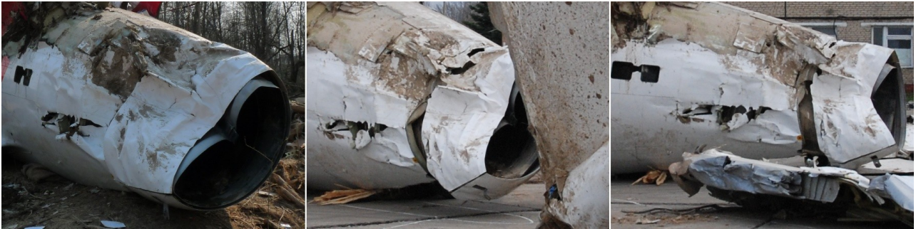
Fig 5: An urban legend presented to the European Parliament: “deformation of aircraft tail has been 'repaired' even before it was moved to storage site”. Deformed engine #2 exhaust nozzle seen on photos from the crash site (left) and storage site on the Smolensk Severny aerodrome
