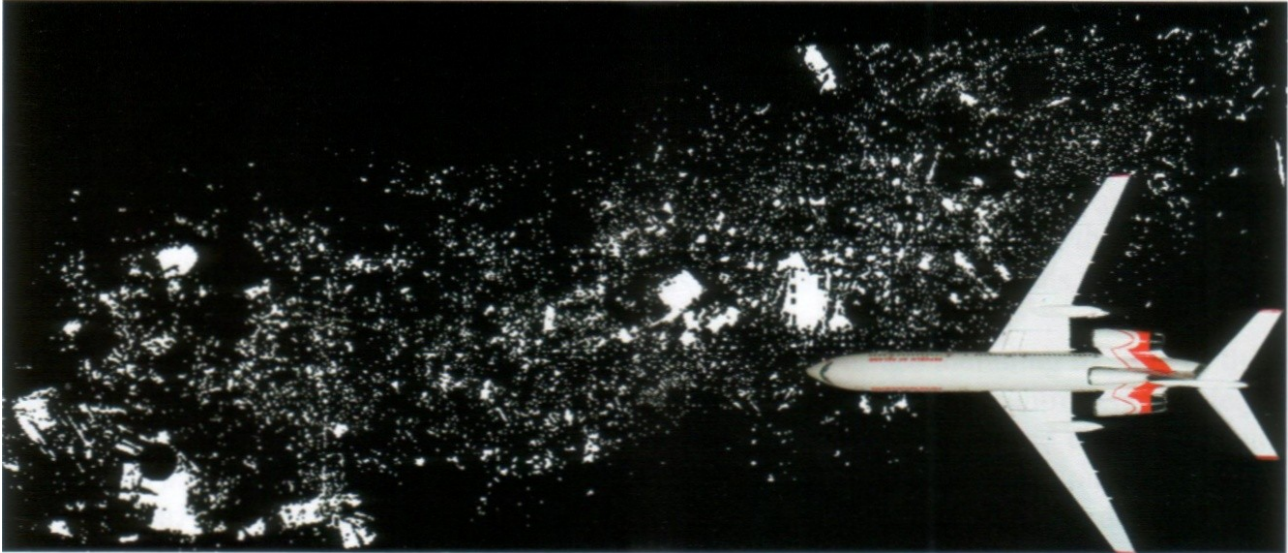
Fig 7: Elongated shape of the main debris field is consistent with shallow impact with ground. Narrow width contradicts the explosion theory. Point of the first impact is just outside the top-right corner of the picture.
