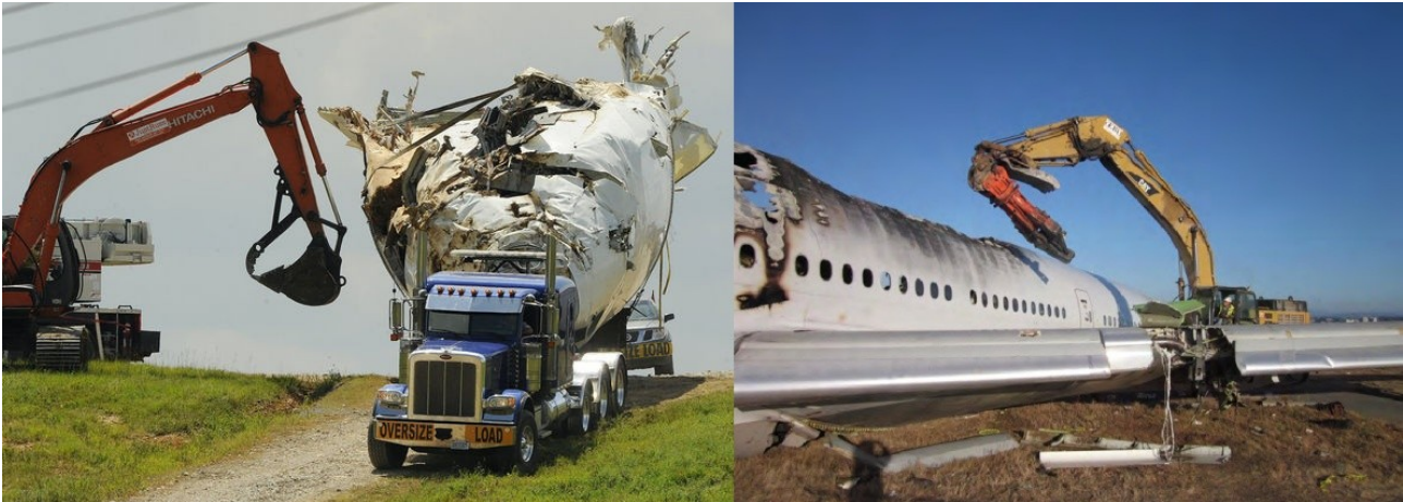
Fig 1: Heavy equipment used to remove aircraft wreckage. Left: Birmingham-Shuttlesworth, Alabama UPS 1354 crash (Source: al.com), Right: San Francisco, California Asiana 214 crash (Source: nycaviation.com)
