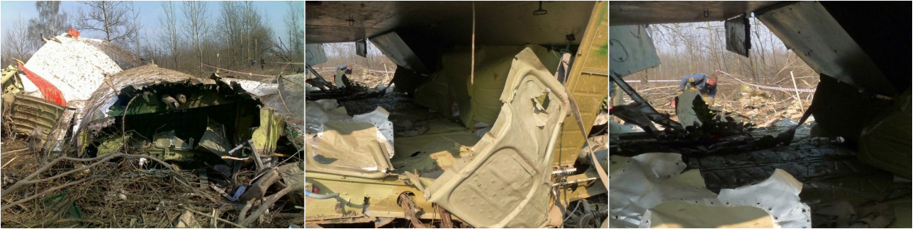
Fig 3: A look inside the cargo hold reveals perfectly flat ceiling (now at bottom) being also the cabin floor, that would be buckled or destroyed in case of explosion in the fuselage.
