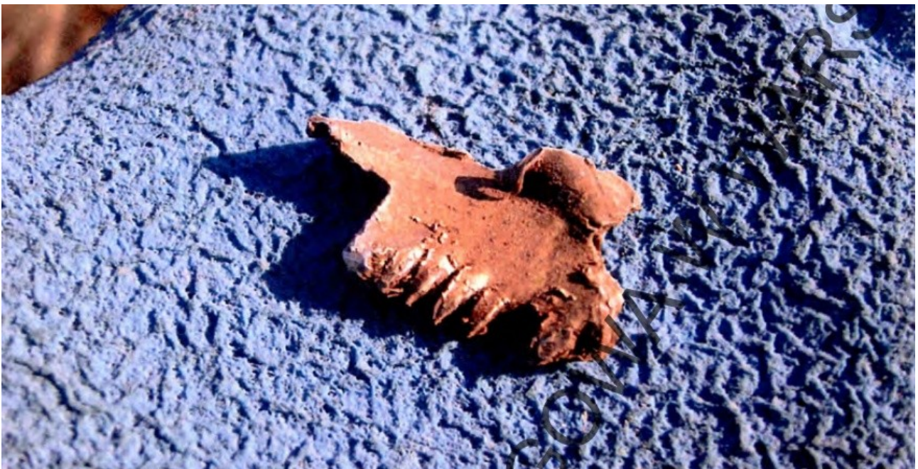
Fig 6: Marks left by tips of rotating turbine blades on a small metal fragment suggest it has been ingested by one of plane's engines – photo from the Archeologists' Report
