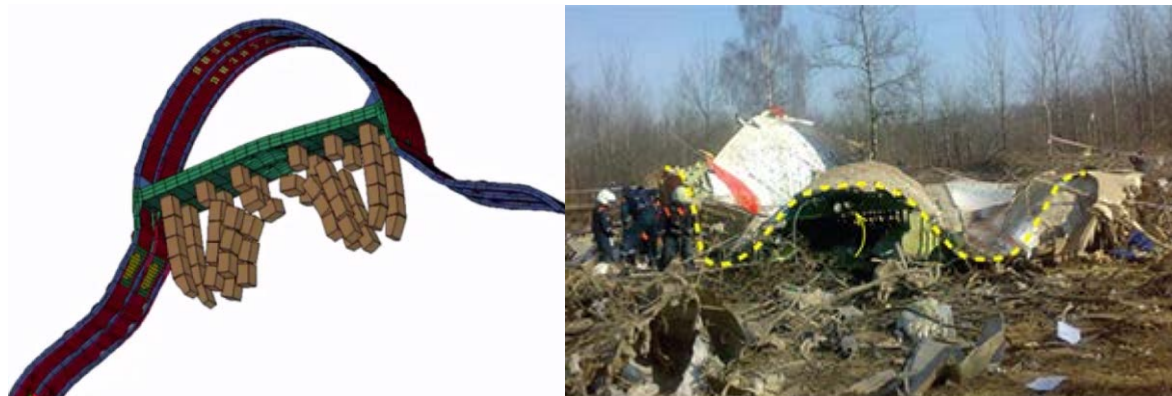
Figure 29. Left - Internal explosion in fuselage - dr. Szuladzinski LS-Dyna simulation. Right - A part of the fuselage inverted and opened up (yellow line and arrow).
