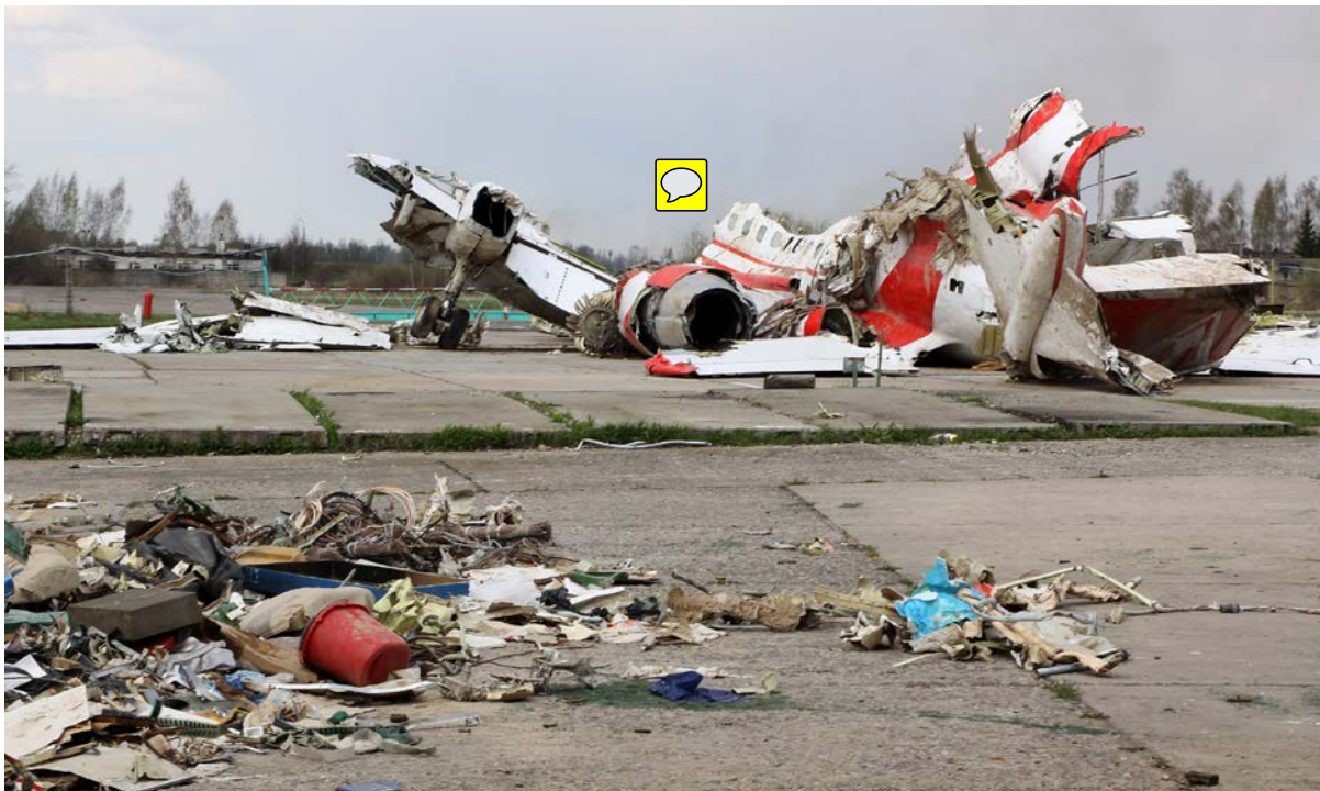
Figure 13. Largest airplane parts on the concrete pavement after transportation from crash site.
