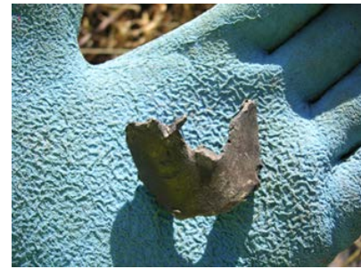
Figure18. Example of a burned metal piece of debris found in front of main crash site. Appendix XI.
