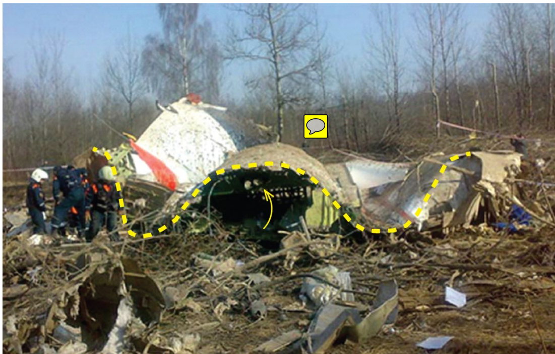
Figure 14. A part of the fuselage inverted and opened up (yellow line and arrow). Appendix VIII.
